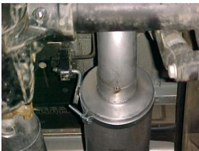
SLIDE MUFFLER #C ONTO HEADPIPES 1-1/2" TO 2". USE A JACK STAND TO SUPPORT MUFFLER.
