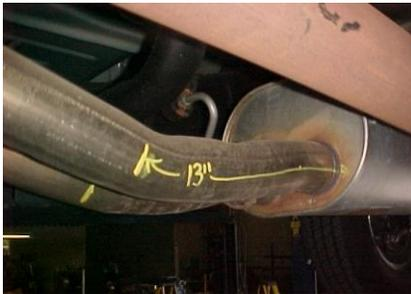
**TO REMOVE STOCK EXHAUST, CUT 13" FROM THE FRONT OF THE MUFFLER,** MEASURE TOWARDS THE FRONT OF THE VEHICLE. LEAVE ALL RUBBER GROMMETS ON THE HANGER. USE WD-40 TO AID IN THE REMOVAL OF EXHAUST AND HANGERS.
